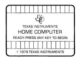
1. Turn the computer ON and wait for the master title screen to appear. Then slide the module into the slot on the console.
